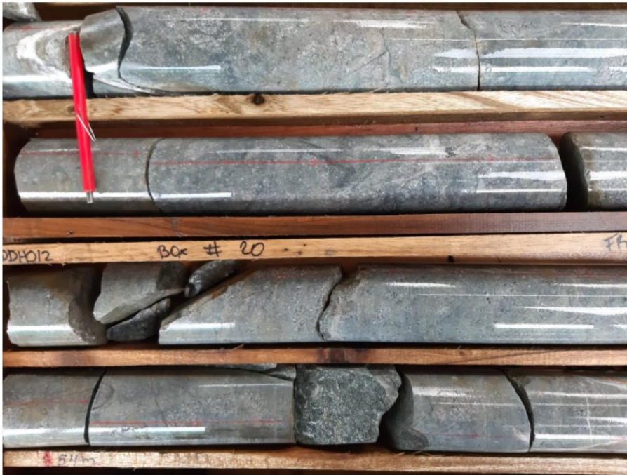
Photo 1. CHDDH12 core 50-54m. Fine grained diorite with fragments of Montana Diorite. Note the black patches and stringers are of secondary magnetite disseminated and in veinlets with secondary K-feldspar halos.
