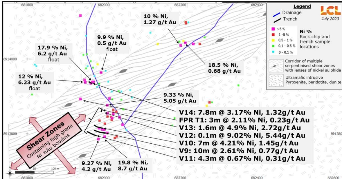
**Figure 2:** Veri Veri nickel prospect. A corridor of shear zones, ~200m wide and open along strike, has been mapped containing boudins of very high-grade Ni ± Au mineralisation. The high grade and volume of boudins, and repetitive nature of the shear zones, provides the potential to 'bulk up' to grades of interest, as evidenced by assays from the numerous trenches across the corridor<sup>3</sup>.
