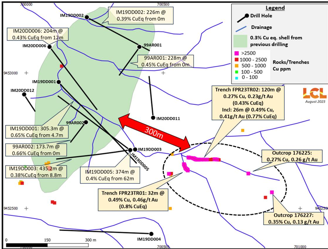
**Figure 4:** Trenches assay results and outcrop grab samples from the recent field campaign at Imou. The green zone is the extent of the 0.3% CuEq shell defined from historical drilling. CuEq calculations are based on US\$3/lb Cu, US\$1,400/oz Au with no allowance for metallurgical recovery<sup>7</sup>.
