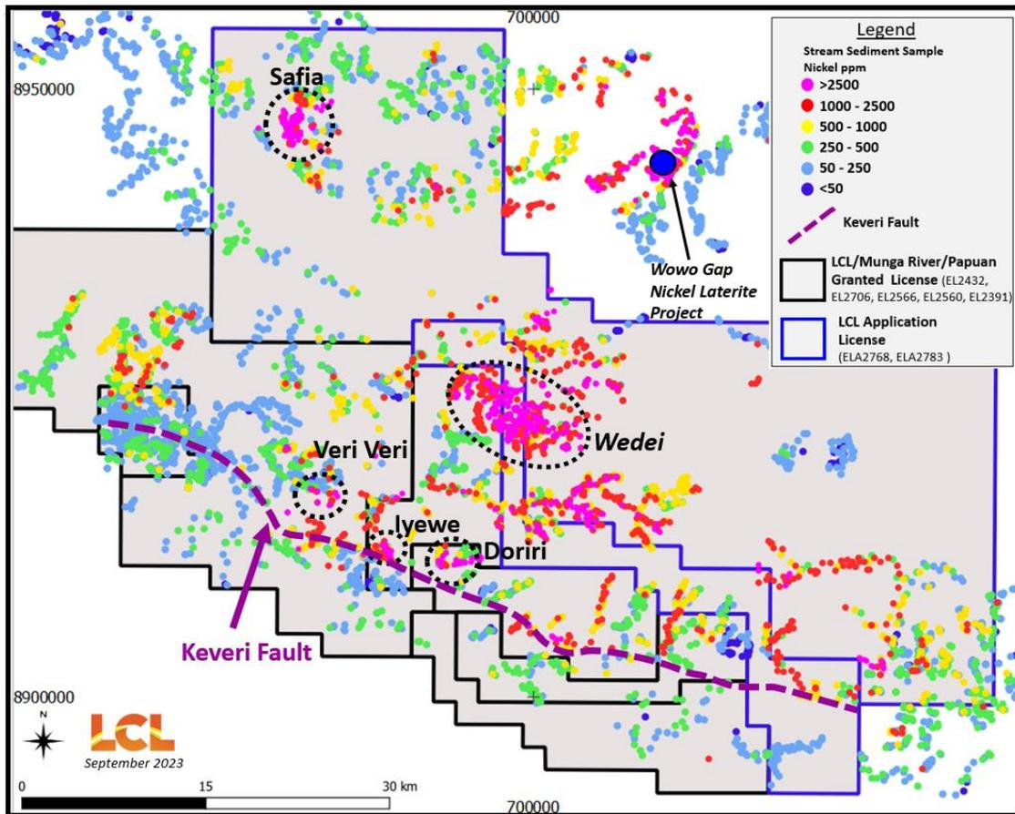
**Figure 3:** LCL's 3,400km<sup>2</sup> nickel exploration portfolio includes multiple nickel targets. Figure shows stream sediment geochemical assays and LCL's exploration licences and applications.
