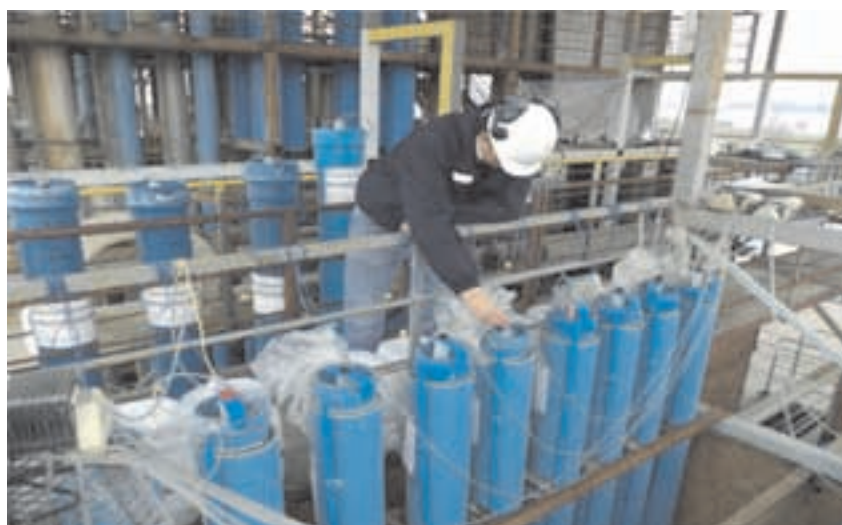
Figure 10: Checking the flow rates at the top of the 6 metre columns, SGS laboratory, Santiago, Chile.
