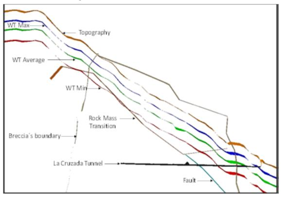
Modeling of the phreatic surfaces from the geotechnical bore holes was undertaken, at maximum, minimum and average level. These have been triangulated in a 3D model, obtaining 3 surfaces representing the maximum, minimum and average water table levels.
