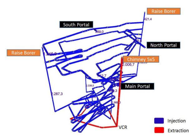
Circuit of injection/extraction ventilation flows (blue - fresh air, red - extracted air)
