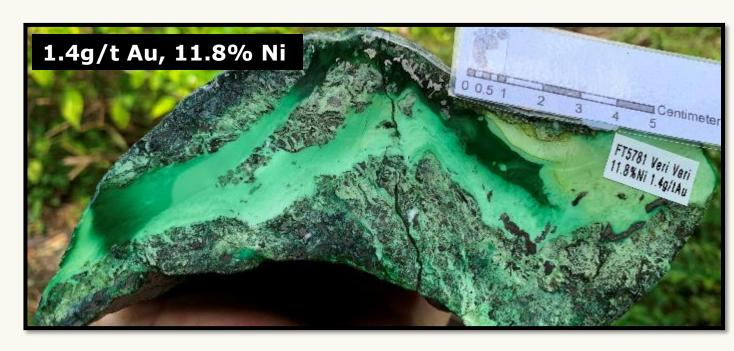
Veri Veri float sample of Ni mineralisation including garnierite
