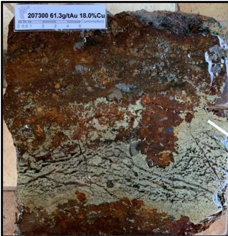
Photo 2: Left - Polished sample from Leah's Lode grading 61.3g/t Au and 18.0% Cu 1 taken ~2m from Leah's Lode Trench FPR TR4 (photo right) which included 8m @ 11.5g/t Au, 2.6% Cu and 24g/t Ag.
