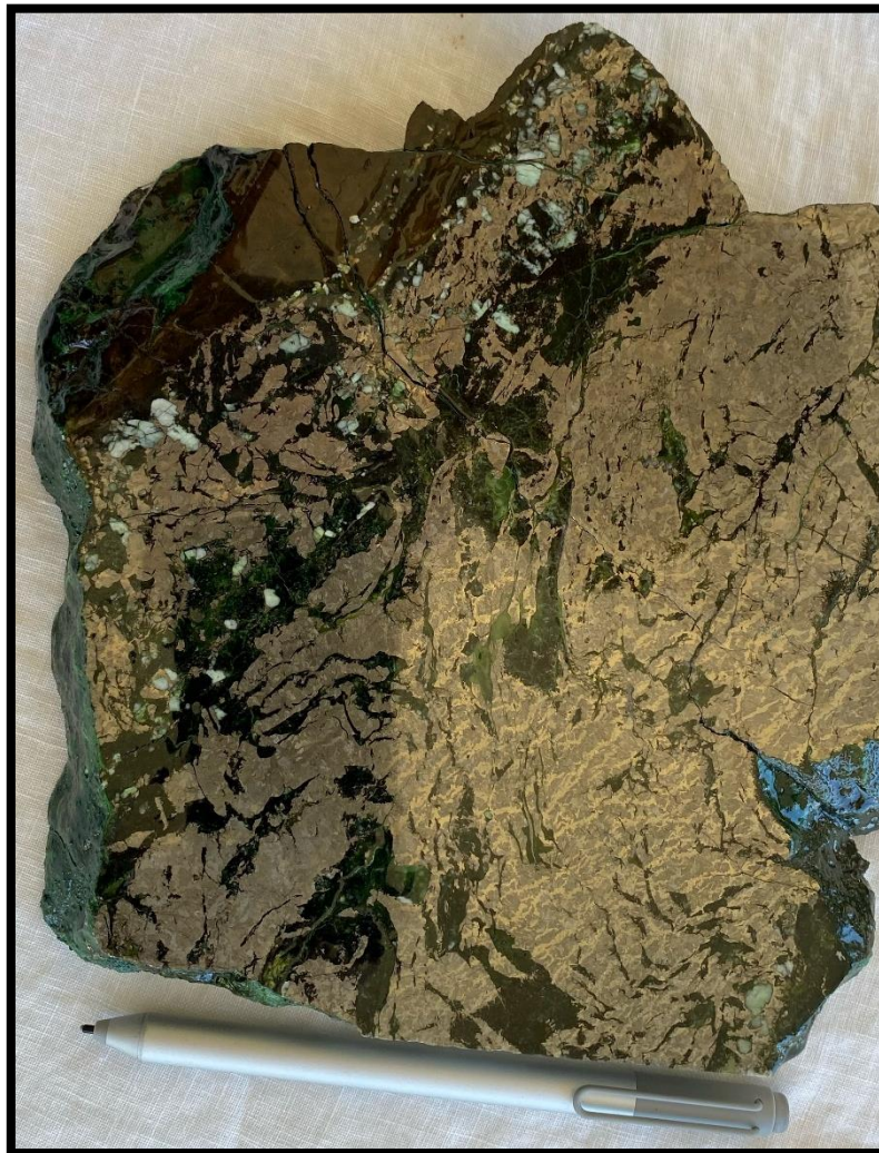
Plate 1: Rock chip outcrop sample 176415 returned 15.78% Ni from composite sample 60cm wide. The polished sample of representative semi-massive nickel sulphide mineralisation is primarily composed of heazlewoodite and serpentine.
