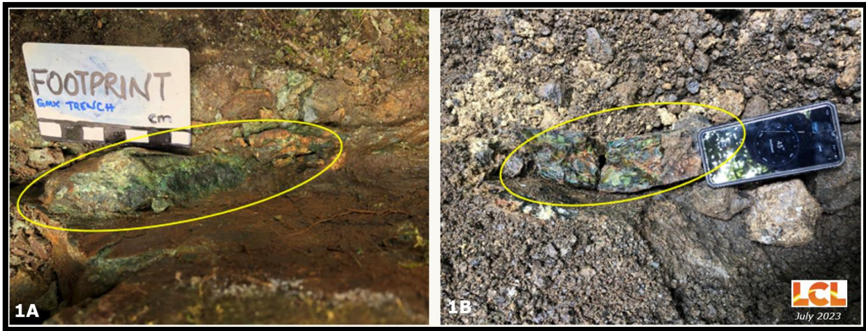
Plate 1: Examples of in-situ boudins of high grade nickel sulphide exposed in pits/trenches. Plate 1B sample 176019: 13.4% Ni, 5.4g/t Au 6 - 10cm x 30cm boudin of nickel sulphide, garnierite, magnetite and trace molybdenite hosted in a shear striking 050 degrees.
