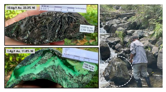
**Plate 1**: Veri Veri creek float samples include massive nickel sulphide minerals (heazlewoodite, millerite, pentlandite) and nickelbearing silicates including serpentinite and garnierite. Photo Right: boulder in creek from which grab sample top left was taken<sup>10</sup>.
