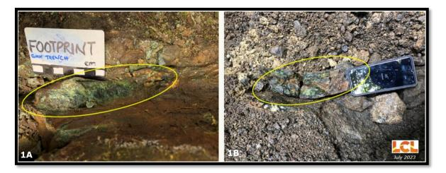
**Plate 2:** Examples of in-situ boudins of high-grade nickel sulphide exposed in pits/trenches. Plate 1B sample 176019: 13.4% Ni, 5.4g/t Au<sup>4</sup> - 10cm x 30cm boudin of nickel sulphide, garnierite, magnetite and trace molybdenite hosted in a shear striking 050 degrees.
