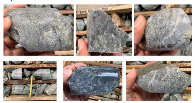
**Photo 3 a to f:** CHDDH006 drill core from ~40m downhole showing A-type quartz stockwork fragments in the intercepted magmatic breccia. Note the different A-type veinlets, granular quartz, banded quartz, smoked quartz and sinuous quartz veinlets with strong K feldspar-biotite-magnetite alteration.
