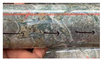
**Photo 1a**. CHDDH009 drill core from ~333m showing the early diorite with potassic biotite-magnetite-K feldspar alteration.<sup>1</sup>
