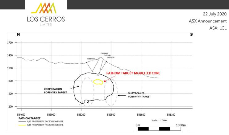
**Figure 4:** Cross section projection showing location of Fathom target in relation to the 2019 drilling program holes and the two porphyry targets established from other methods. See Figure 3 for north-south location of cross section.
