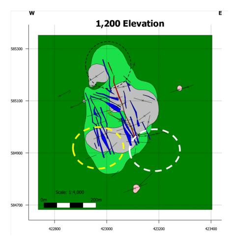
**Figure 2:** Modelling of high grade distribution has revealed three regions justifying further testing, two associated with the potential extensions of shoots - white dashed circle at depth and black dashed circle near surface in the above plan. The depth extent of white-grey breccia (yellow circle) has not been tested and is the third target.
