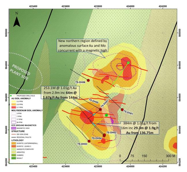
**Figure 5**: Tesorito is an at-surface gold mineralised porphyry system. The Company's first hole of the pending drill program will further explore the southern anomalous zone that has already delivered impressive results. The Company is also developing its drilling strategy for the northern anomalous zone defined here by gold and strong molybdenum assays in soil over a magnetic high.
