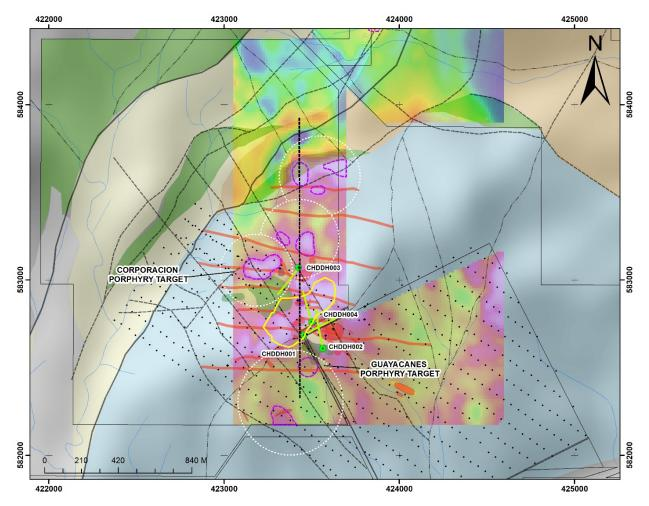
**Figure 3:** Chuscal plan view showing the Fathom target (yellow outline) in relation to LCL drill holes CHDD001-004 (too shallow to intersect Fathom target) and existing porphyry targets (dotted white circles) established from other data, over background magnetics. Purple bordered shapes are magnetic highs of interest. Note the north-south orientation of targets, this orientation extends northward to align to the Tesorito Prospect located 1.5km to the north.
